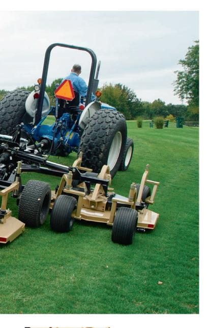
Anti-scalp rollers on nose and trailing edges of decks protect the deck as well as the turf.
